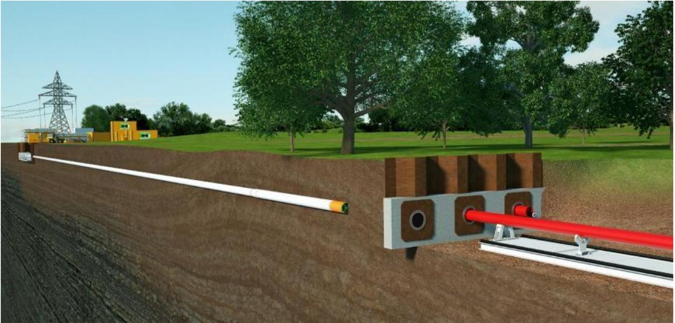
Picture 2. The E-Power Pipe method for trenchless installation of underground cables
